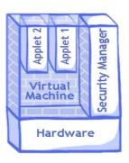
The figure above shows the two main (high level) components of the QX operating system, the security manager and the virtual machine. Documents [25], [20] and [21] and give an overview of QX, describe the QX security manager and the QX virtual machine respectively.
